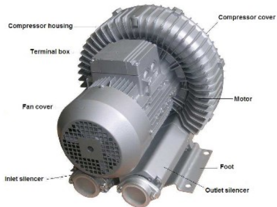
Fig. 1: Side channel blower parts
