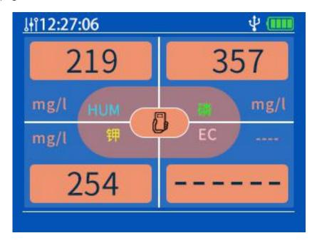
Short press "right key" or "bottom key" in multi-joint interface, automatically jump to single data display interface, single data display interface will only display a certain kind of data.
