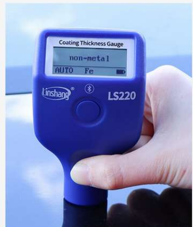
LS220 Car Paint Meter tests non-metal car body
