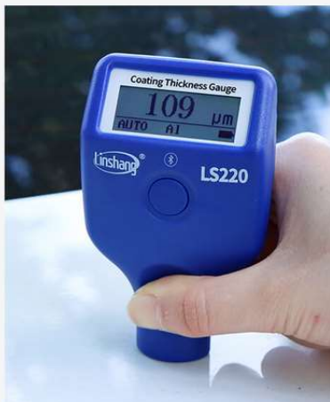
LS220 Car Paint Meter tests aluminum car body
